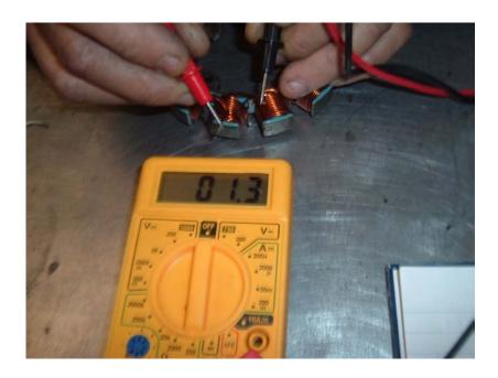
Figure 4 – Circuit identification
