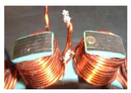
Figure 5 - Twisted wire connection
