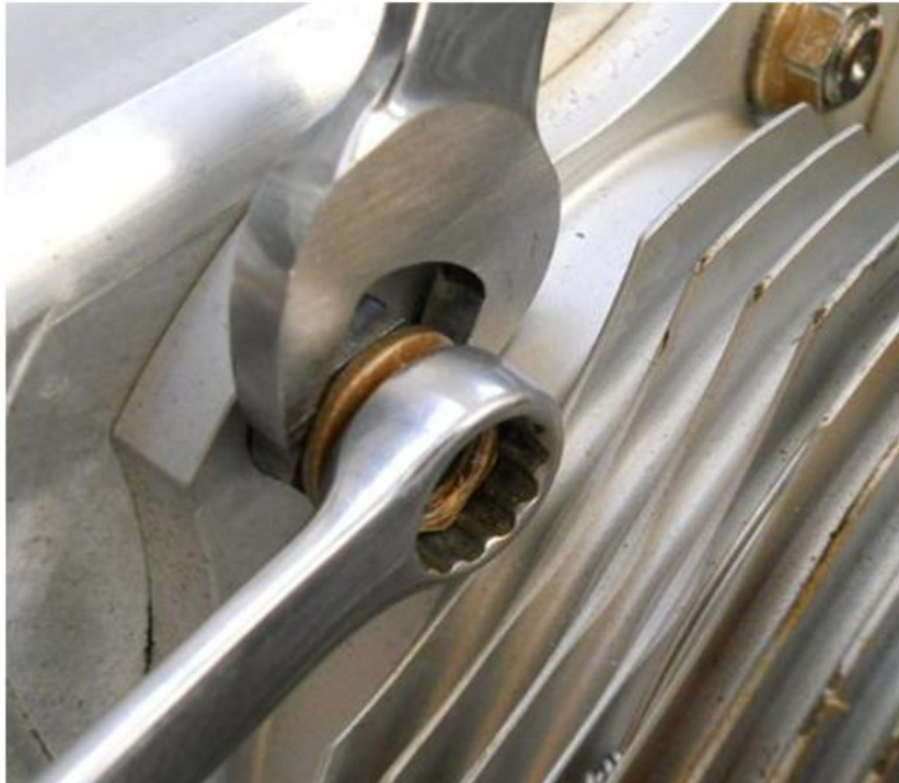
Figure 10 - Using lock nuts to remove the second reduced hex.
