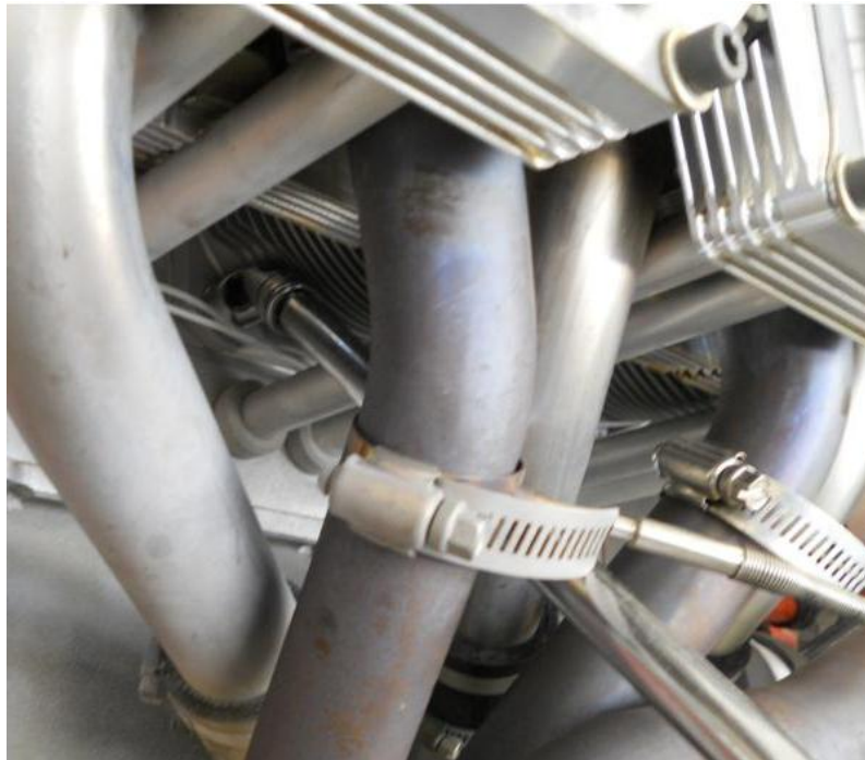
Figure 9 - Accessing concealed nuts
