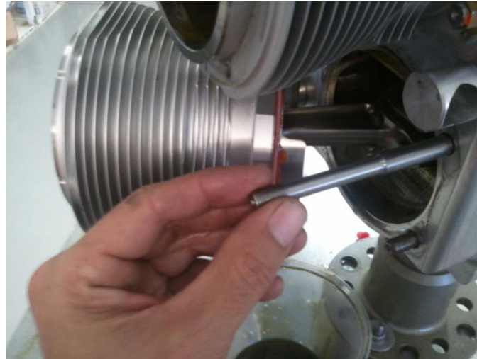
Figure 5 – Replacing Through Bolts
