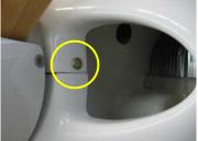
Starting with the bottom cowl, remove one 6G stainless steel screw at a time and drill the hole out to 3/16°, then drill the 3 holes in the top cowl to 5/16°.
