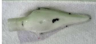
When the Araldite/flock has cured, heat and remove the screws, mix a small batch of resin and apply a single layer of AF303 glass fibre cloth on the inside of the cowl over both sides and across the rear of the scoop. Leave overnight to cure.
