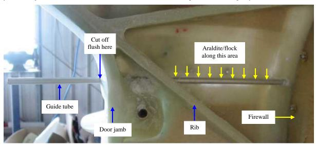
Continue to drill through the rib until the guide tube can be pushed all the way from the door jamb and through the firewall.
