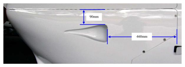
Assemble the duct with 5-minute Araldite. Hold the scoop on the outside of the cowl in the position as shown above, keeping the rear edge of the scoop at right angles to the hinge line and mark around the outside of the unit and then make a second line inside the first about the size of the actual opening.
