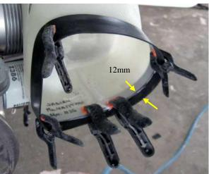
Remove the top cowl and mark the front of the ram air ducts 10mm back from the inside of the bottom cowl as shown above left.
