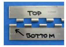
Assemble each hinge pair by sliding the long hinge pin through the full length of the hinge. Note that the hinge pin is much longer than the hinge – do **not** trim the hinge pin to length! The extra length will be used when the hinge pin is fitted through from the door jamb and into the hinge later in this step. Put a cloth tape flag on the exposed end of the hinge pin to prevent possible accidents.
