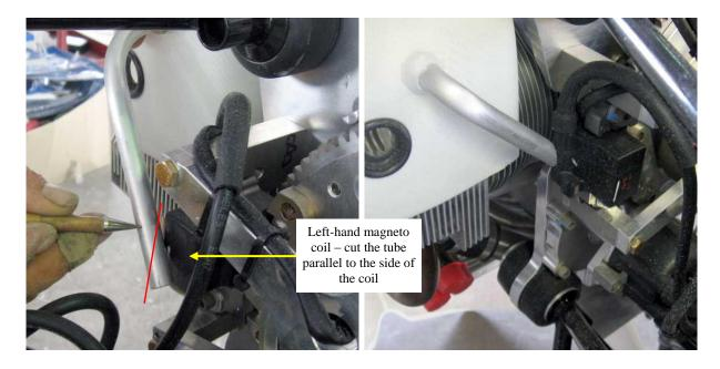
Starting with the left-hand duct, drill a  $\frac{1}{2}$ " hole at the top centre rear of the duct and slip the curved aluminum tube into place until the mark on the tube reaches the duct. Aim the lower end of the tube at the centre of the left-hand magneto coil, mark the tube at an angle parallel to the side of the coil, remove the tube and cut along the mark. Shorten the top end of the tube as required – it should fit about  $1\frac{1}{2}$ " to 2" (40-50mm) inside the duct.
