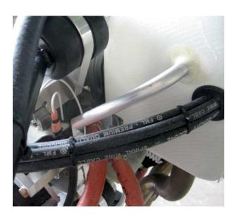
This completes the *Pre-Paint>Fuselage>Firewall forward>Fit ram air cooling ducts* task.
