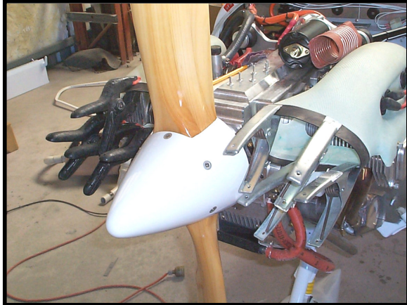
Clamp rubber while rubber is being glued.
