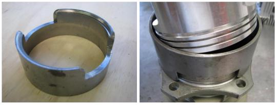
Figure 18 - Piston & Ring Installer
