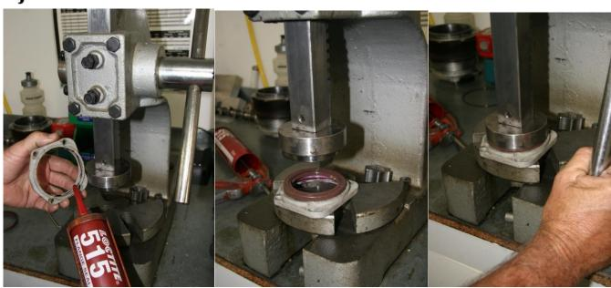
Figure 201 – Fitting Seal To Housing
