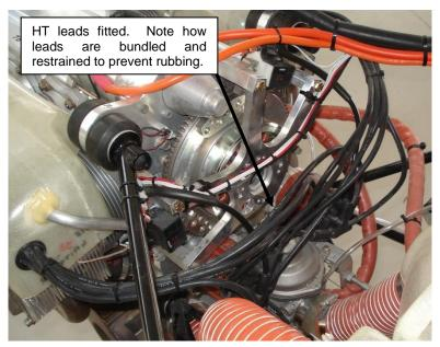
Figure 200 - HT Leads Fitted To Engine
