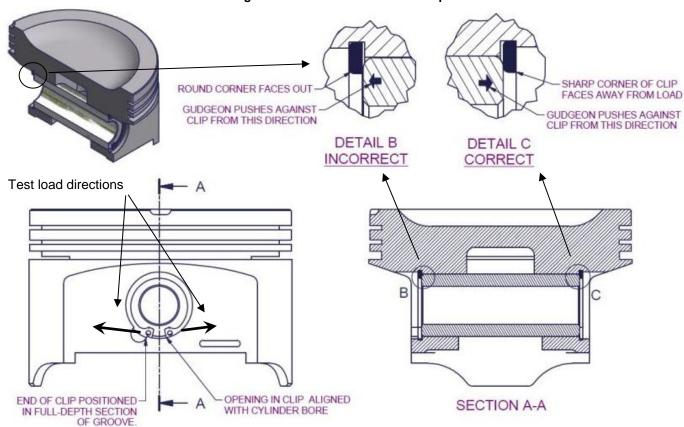
Figure 136 - Clip Installation Detail
