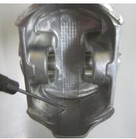
Figure 131 - Thrust Direction Markings For Pistons
