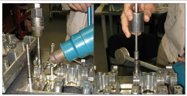
Figure 73 - Removing Studs and Dowels from Crankcase
