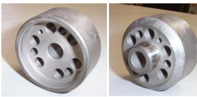
Figure 214 - Drilling Fixture - Crankshaft Side on Left, Flywheel Side On Right
