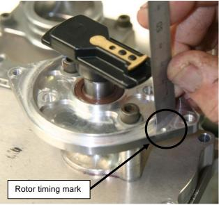
Figure 176 - Setting Distributors, Checking Rotor Position
