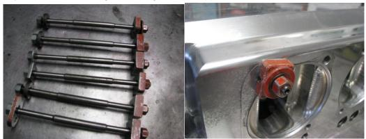
Figure 32 - Crankcase Dry Fit Through-Bolts and Nuts
