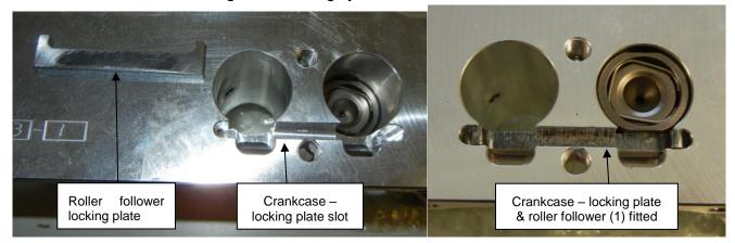
Figure 187 - Crankcase & Locking Plate
