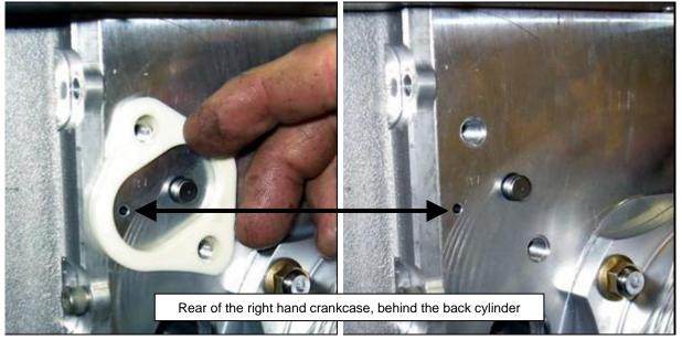
Figure 70 - Fuel Pump Oil Drain
