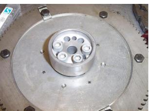
Figure 218 - Aligning Guide & Fitting To Flywheel.
