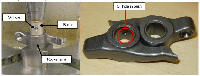
Figure 99 - Fitting Rocker Bush
