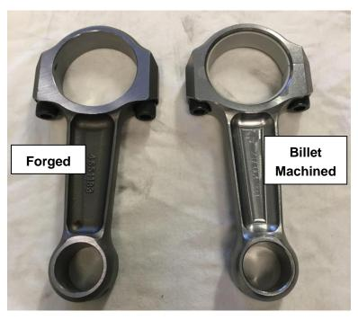
Figure 122 - Forged conrods vs Billet machined conrods
