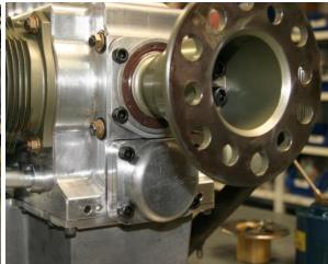
Figure 206 - Engine Turning Tool, Installed Oil Pump
