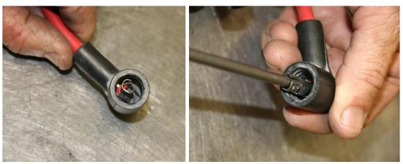
Figure 110 – Adjusting High Tension Lead Caps
