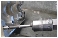
A tool which clamps onto the tip thread of the stud, holding it tightly and allowing the stud to be screwed out of the crankcase.
