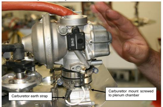
Figure 197 - Fitting Carburettor
