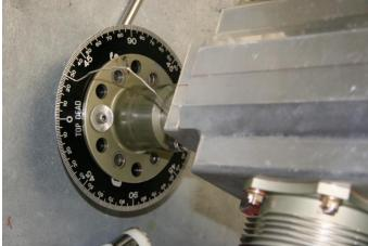
Figure 175 - Fitting Distributor Case & Setting Timing
