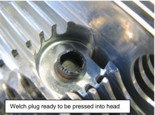
Figure 146 - Cylinder Head Welch Plug & Lube Tube Installation.
