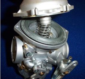
Figure 113 - Disassembling Carburettor #1
