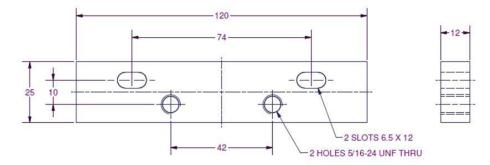
Figure 11 - Dimensional Details For Lifter Tool
