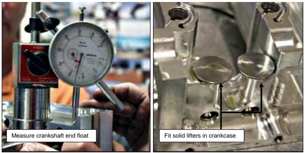
Figure 128 - Checking Crankshaft End Float, Installing Solid Lifters
