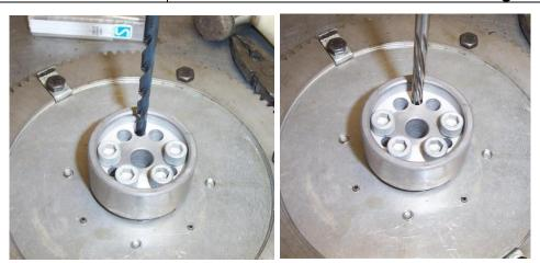
Figure 219 – Drilling & Reaming Flywheel – ILLUSTRATION ONLY.
