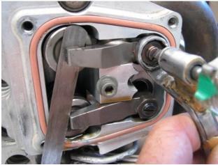
Figure 194 - Valve Clearance Adjustment (Solid Lifter)
