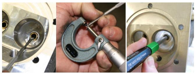
Figure 91 - Measure Guide Wear (Telescopic Gauge Left & Middle, Go-No-Go Gauge Right)
