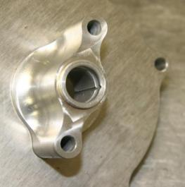
Figure 153 - New Distributor Shaft Bush Fitted - nopic x 1
