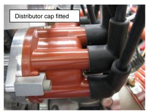
Figure 185 - Distributor Cap Installation
