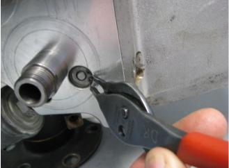
Figure 207 - Lapping Oil Pressure Relief Valve
