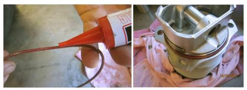
Figure 159 – Applying Sealant and O-Ring to Cylinder Base
