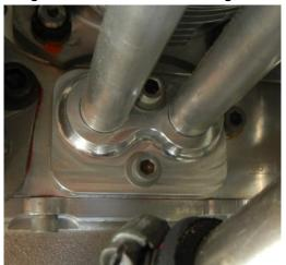
Figure 188 - Oil Return Manifold Fitted
