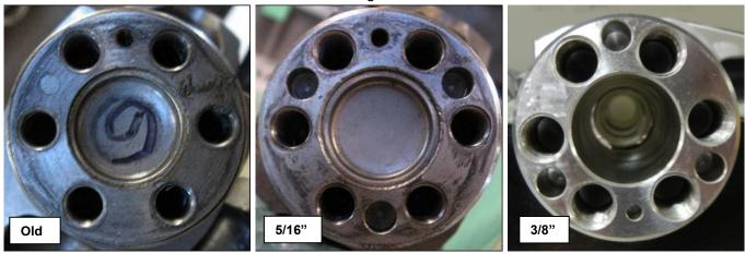
Figure 64 - Crankshaft End Detail (Dowel Holes)
