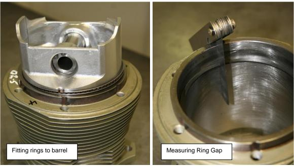
Figure 138 - Checking Piston Ring Gap
