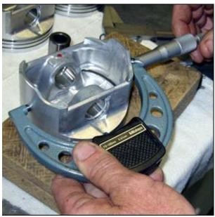
Figure 85 - Measuring Cylinders & Pistons
