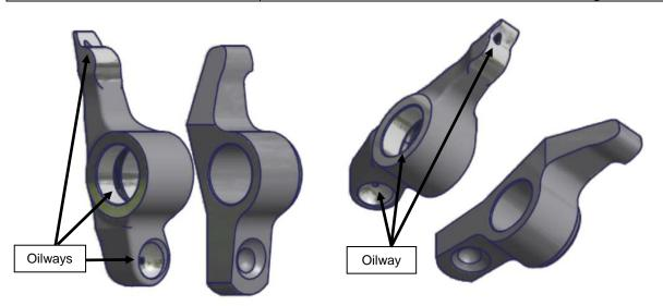
Figure 100 - Solid VS Hollow Valve Rockers
