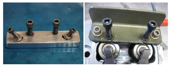
Figure 10 - Valve Compressor / Lifter Bleed Tools
