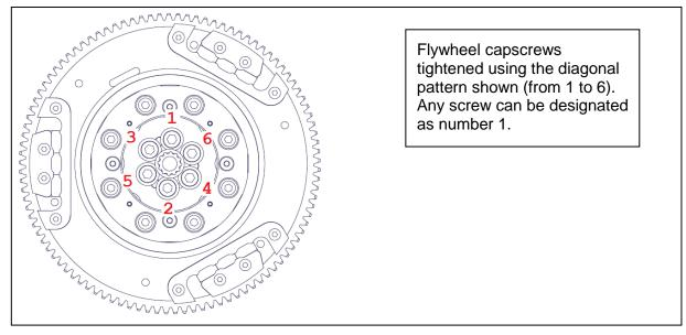
Figure 181 - Flywheel diagonal tightening pattern
