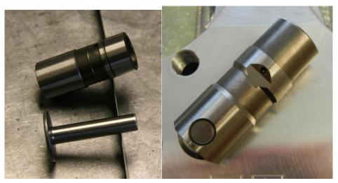
Figure 75 - Hydraulic Lifter (top left), Solid Lifter (lower left), Roller Follower (right)
