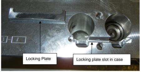
Figure 58 - Crankcase & Locking Plate
