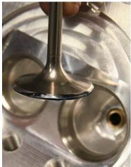
Figure 93 - Recessed Valve Seat, Valve Being Cut
