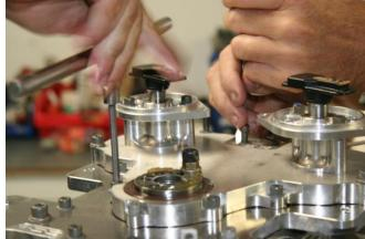
Figure 177 - Checking Rotors, Tightening Distributor Case
