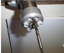
Figure 217 - Drilling & Reaming Crankshaft - ILLUSTRATION ONLY.
