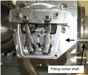
Figure 191 - Fitting Rockers #2
