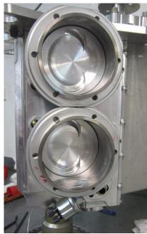
Figure 132 - Installation of Pistons With Valve Relief
