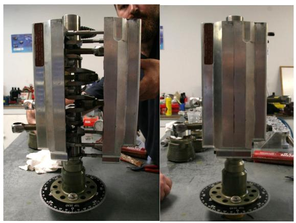
Figure 157 - Fitting The Second Case Half
