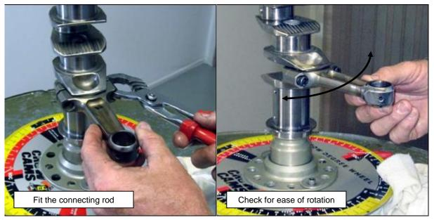
Figure 121 - Fit Connecting Rods
