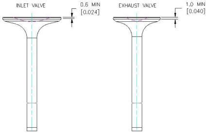
Figure 88 - Valve Measuring
