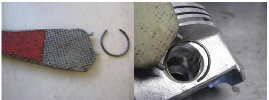
Figure 134 - Fitting Wire-Type Piston Circlips
