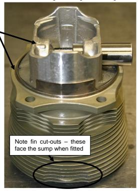
Figure 141 - Piston / Ring / Cylinder Assembly
