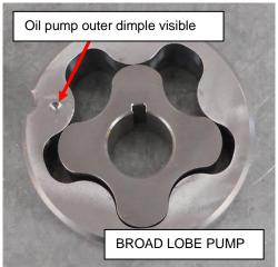
Figure 205 - Fitting Oil Pump & Port Plate
