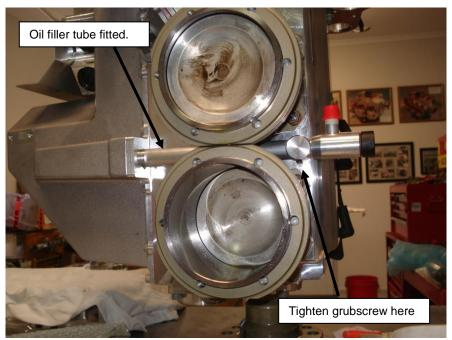
Figure 171 – Oil Filler Tube Installation
