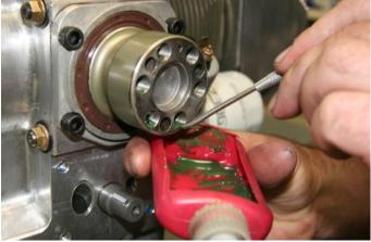
Figure 203 - Preparing To Fit Propeller Flange
