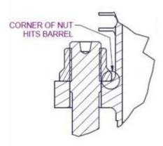
Figure 142 - Through Bolt Nut Installation Detail
