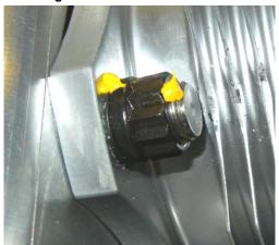
Figure 163 - Torque Seal Applied
