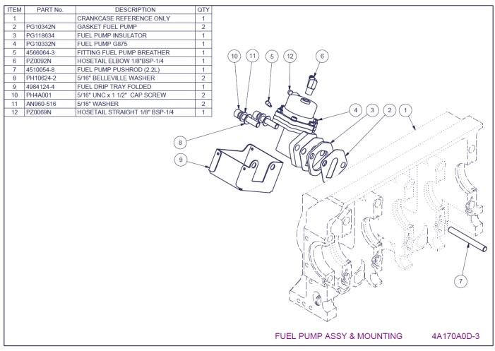
Figure 155 - Mechanical fuel pump installation
