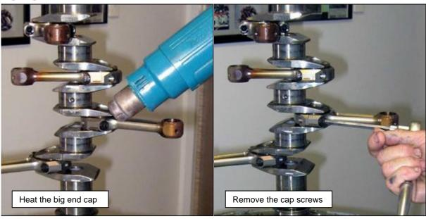
Figure 61 - Remove Con-Rods
