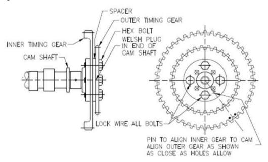
Figure 129 - Cam Timing Gear Assembly
