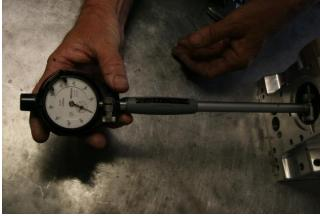
Figure 72 - Measuring Crankcase Bearing Tunnel
