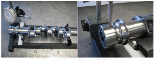
Figure 26 - Crankshaft Run-Out Test Bed
