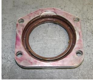
Figure 202 - Front Seal Housing Ready To Fit
