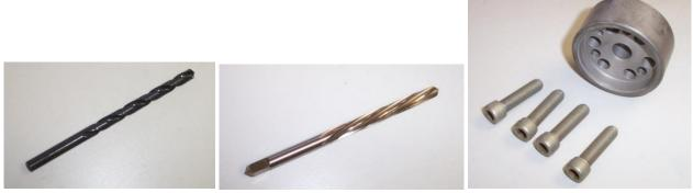
Figure 215 – 15/64" Drill (Left), 6mm Ream (Centre), UNF Cap Screws (Right)
