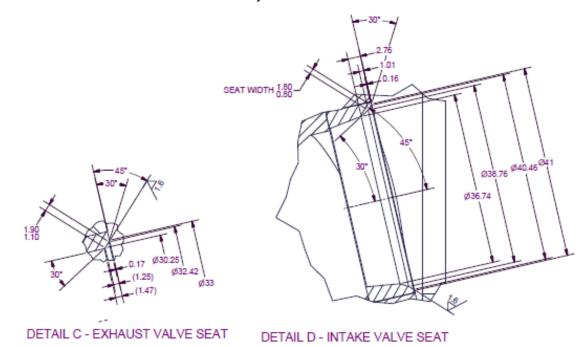
Figure 92 - Valve Seat Geometry
