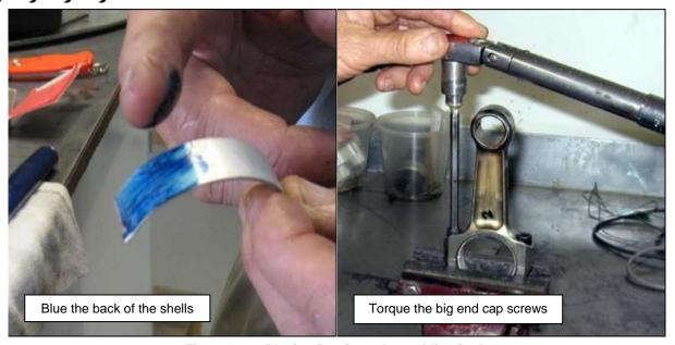
Figure 119 - Blueing Bearings, Assembling Rods
