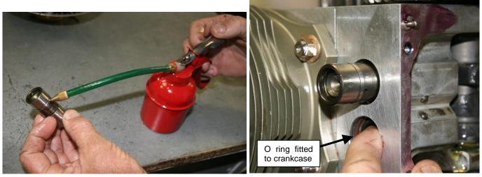
Figure 186 - Fitting Hydraulic Lifter To Crankcase
