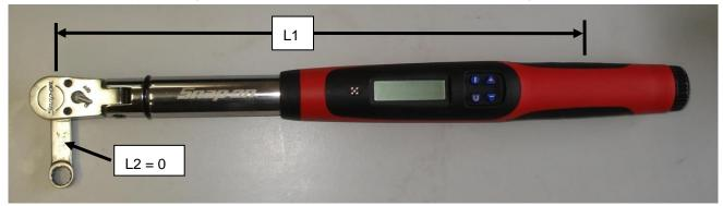
Figure 39 - Torque Wrench & Crowsfoot Adaptor Setting 2
