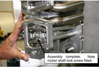
Figure 192 - Fitting Rockers #3
