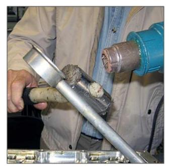
Figure 60 - Remove Oil Strainer
