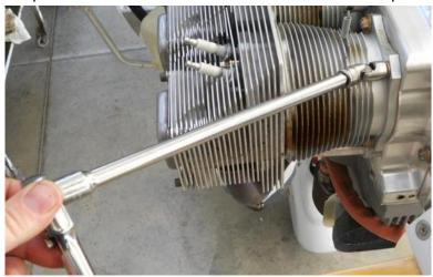
Figure 164 – Universal Joint tool FU14B (FU16B for ½" Socket)
