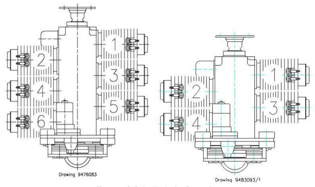
Figure 3 - Cylinder Numbering Convention
