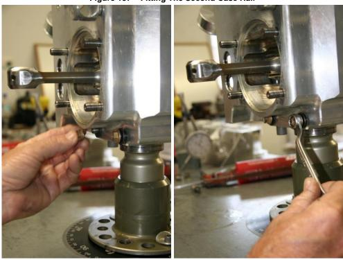
Figure 158 - Tightening The Front Crankcase Studs
