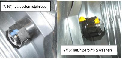
Figure 143 – 12-Point Nuts, 7/16" Hardware (on right)
