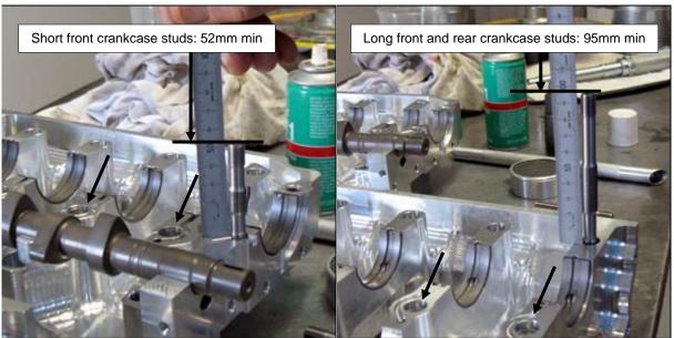
Figure 123 - Crankcase Assembly Preparation
