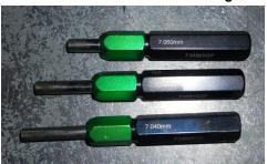
Go-Nogo gauges are used to quickly and accurately check the inner size of a valve guide. Sizes 7.03 / 7.04 / 7.05 / 7.06 / 7.07 / 7.08. Gauges produced by 'Prittie' (www.prittie.com.au) are used in the factory.
