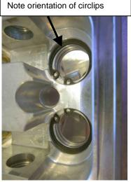
Figure 190 - Fitting Rockers #1
