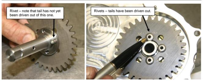
Figure 154 - Assembling Distributor Gear to shaft
