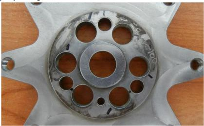
Figure 104 - Damaged Flywheel "Starfish"
