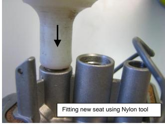
Figure 115 - Fitting New Float Needle Seat
