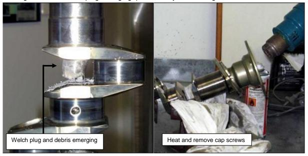
Figure 62 - Welch Plug & Propeller Flange Removal From Crankshaft
