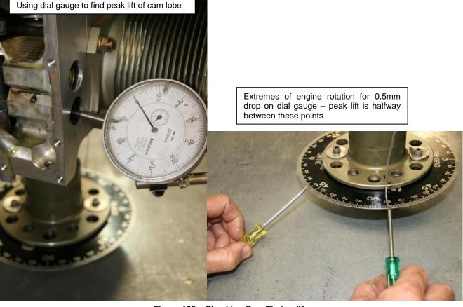
Figure 168 - Checking Cam Timing #1
