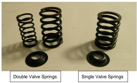
Figure 97 - Double Valve springs vs original single spring
