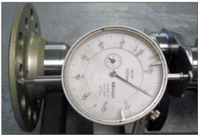
Figure 66 - Crankshaft Measurement
