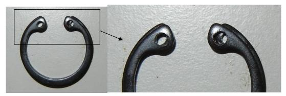
Figure 137 - Over-Compressed and New Clips
