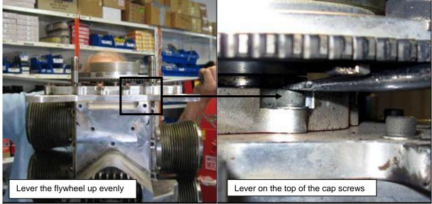
Figure 49 - Removing Flywheel
