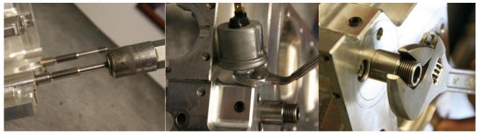
Figure 212 – Stripping Crankcases
