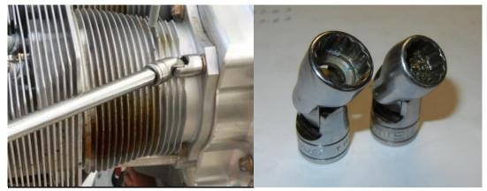
Figure 37 - Universal Joint tool FU14B
