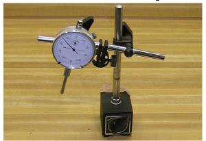
As well as Crankshaft run-in, a dial gauge is also used to locate top dead centre (TDC) in the cylinder.
