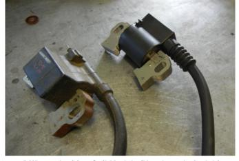
Figure 103 - Different Ignition Coil Models (Honda on Left, Jabiru on Right).
