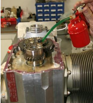
Figure 172 – Sealing Engine Mount Plate
