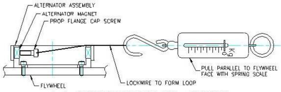
Drawing 9438064/1 MAGNET PULL TEST - ALTERNATIOR
