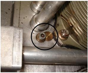
Figure 193 - Rocker Lube (Left) & Crankcase Oil Port Blanking Plug
