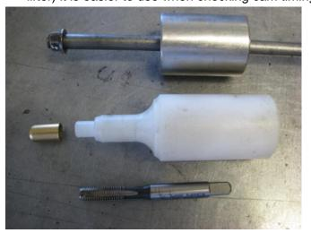
The tap (at bottom) is used to cut a thread into the needle seat (small part, middle-left). The slide hammer (at top) screws into this thread and is used to draw the needle seat out of the carburettor. The nylon driver (in centre) is used to fit the new needle seat to the carburettor body.
