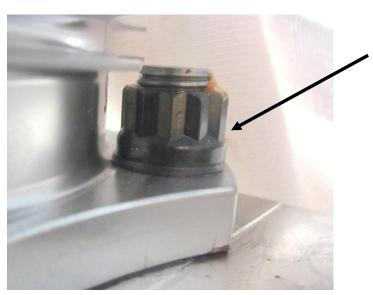
Nut on assembled engine. Note "new type" barrel, small-flange 12-point nut & washer shown.
