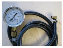
Used during initial engine proof runs and / or running-in. Used as a more accurate gauge to confirm the readings of the standard aircraft oil pressure gauge. Fitting uses 1/8 NPT thread.
