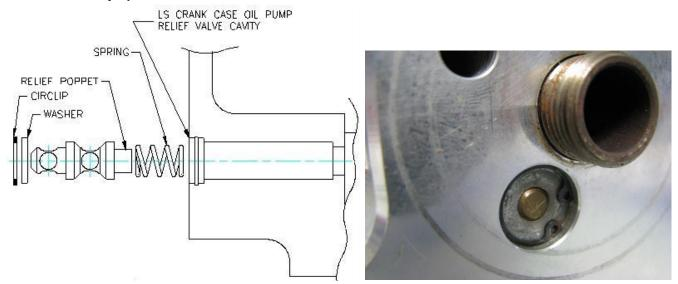
Figure 83 - Oil Pressure Relief Valve
