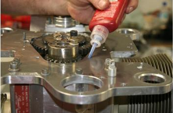
Figure 173 – Fitting Engine Mount Plate
