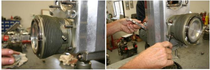
Figure 161 – Fitting Cylinder, Inserting & Tightening Through-Bolts
