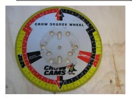
A degree wheel or degree disc – used during engine assembly to check engine timing.
