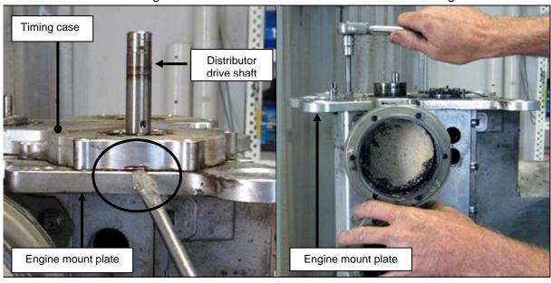
Figure 50 - Remove Timing Gearbox Case
