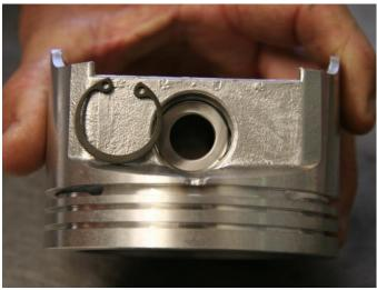
Figure 133 - Fitting Circlip to Piston
