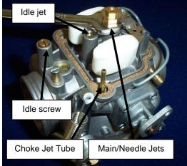
Figure 114 - Disassembling Carburettor #2
