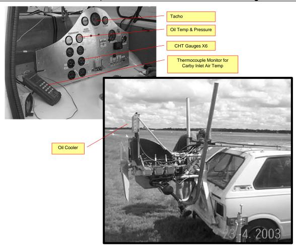
Figure 209 - Engine Ground Running Rig
