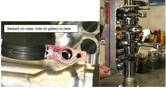
Figure 156 - Applying Sealant to Case, Fitting to Crank
