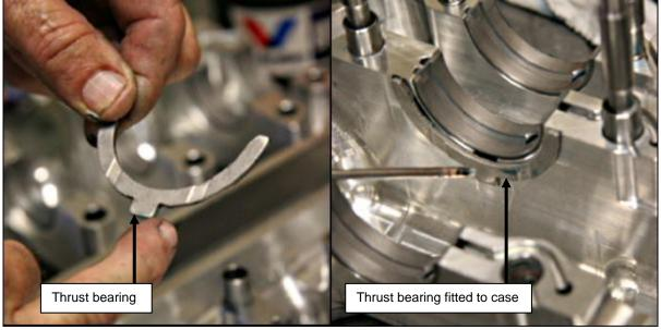
Figure 126 - Fitting Thrust Bearings
