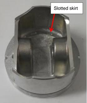
Figure 140 - Split and Slotted skirt pistons
