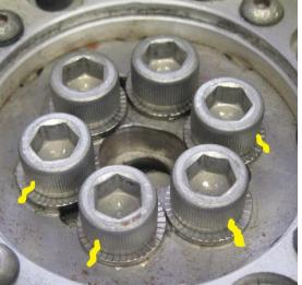
Repeat for the other five screws ONE AT A TIME using the diagonal pattern shown in Figure 181
