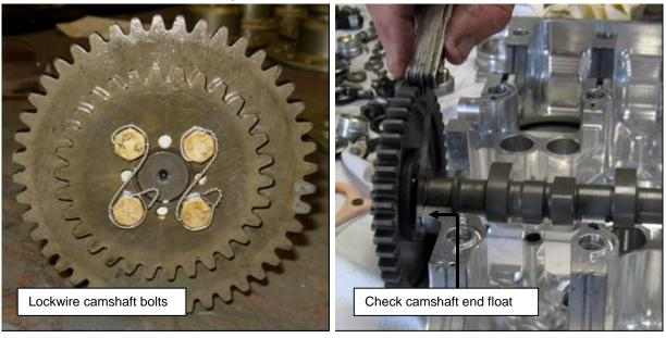
Figure 130 - Assembling Cam & Fitting to Crankcase
