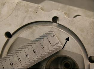
Figure 87 - Cracking Between Valves, Recessed Cylinder Spigot
