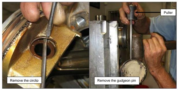
Figure 55 - Remove Pistons
