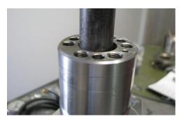
Essentially a long, large punch used to both remove and install the welch plugs from the ends of the crankshaft.
