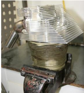
Figure 95 - Valves Assembly, Cylinder Head / Cylinder Lapping
