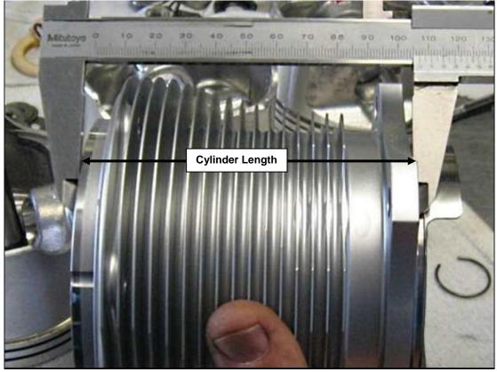
Figure 84 - Measuring Cylinder Length
