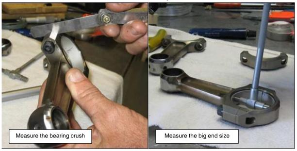
Figure 120 - Measuring Connecting Rods
