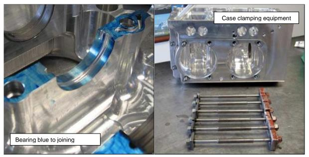
Figure 125 - Crankcase Clamping Preparation
