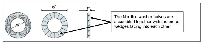
Figure 182 - Nordloc washer halves assembled together
