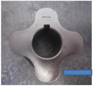
Figure 82: Broad lobe inner gear with line marking.
