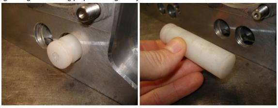
Figure 29 - Cam Timing Tool (Hydraulic Lifter)
