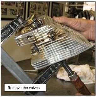
Figure 47 - Cylinder Head Disassembly
