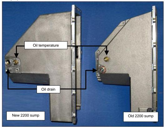
Figure 101 – 2200 Engine Sumps
