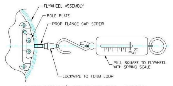
Drawing 9437064/1 MAGNET PULL TEST - FLYWHEEL
