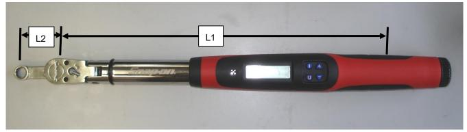
Figure 38 - Torque Wrench & Crowsfoot Adaptor Setting 1
