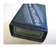
An accurate optical tachometer. Reads directly from reflective strips fitted to the propeller and is used whenever an accurate check of RPM is required. Will usually read propeller RPM in sunlight without reflective strips.
