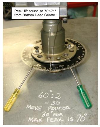
Figure 169 - Checking Cam Timing #2
