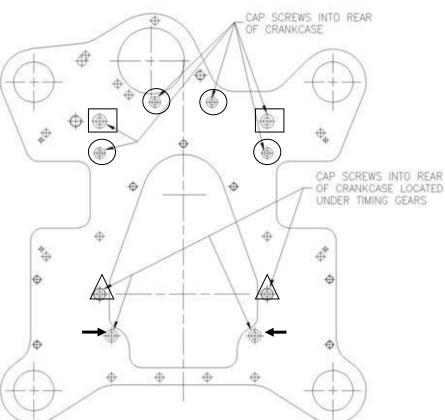
Figure 174 - Engine Mount Plate Screw Locations
