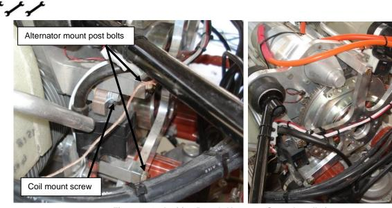
Figure 184 – Ignition Post & Alternator Stator Installation
