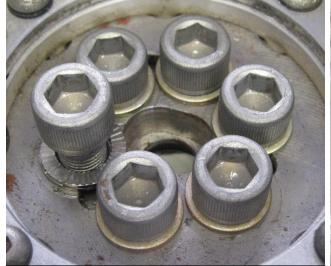
Reinstall capscrew with ONE Nordloc washer pair to **Prescribed Torque** (Table 9) directly. Apply Torque seal, paint pen mark or liquid paper
