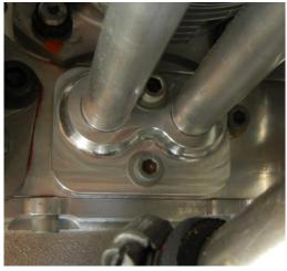
Figure 57 - Oil Return Manifolds
