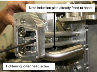
Figure 189 - Applying Thread Lubricant & Tightening Lower Head Screw
