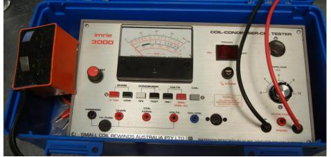
Figure 27 – Ignition Coil Tester
