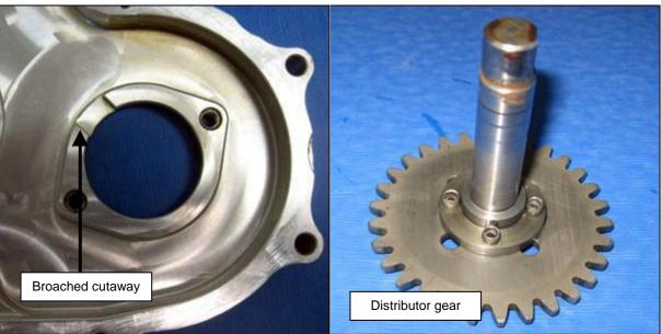
Figure 109 - Distributor Gears & Case
