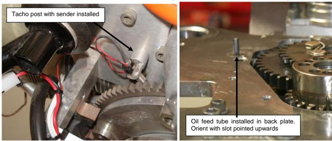
Figure 150 - Installation of Oil Feed Tubes & Tacho Pickup Post
