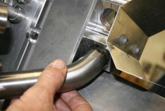
Figure 196 – Fitting Induction Pipes to Plenum Chamber
