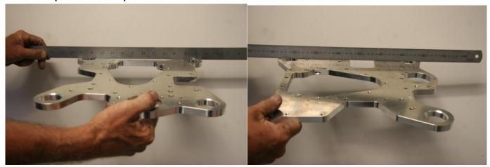
Figure 108 – Checking Engine Mount Plate Trueness
