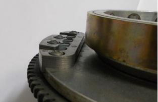
Figure 149 - Laminated Magnet retaining pole plates
