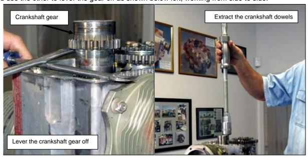
Figure 53 - Removing Crankshaft Timing Gear & Dowels
