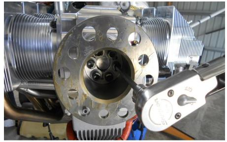
Figure 204 - Installing the Propeller flange
