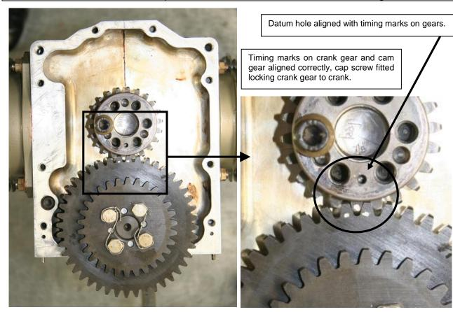
Figure 167 - Setting Cam Timing
