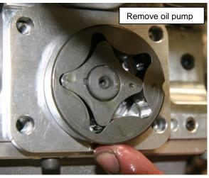
Figure 56 - Front Seal & Oil Pump Removal
