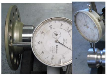
Figure 44 - Measuring Propeller Flange & Crank Run-Out
