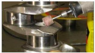
Figure 67 - Radius Crank Centre Holes
