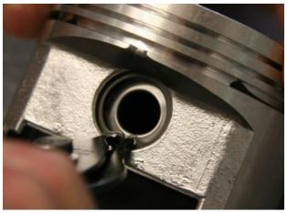
Figure 21 - Standard Circlip Pliers
