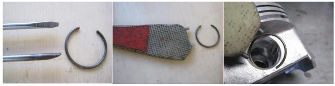
Figure 20 - Piston Circlip Remover and Installer
