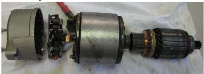
Figure 106 - Typical Disassembled Starter Motor
