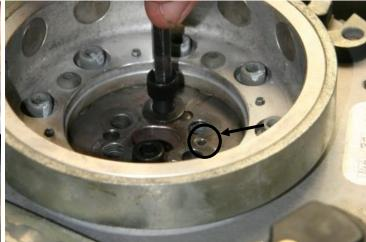
Figure 180 - Flywheel & Crank Timing Marks
