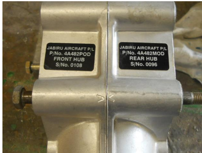
Figure 4 - Propeller hub indexing arrows
