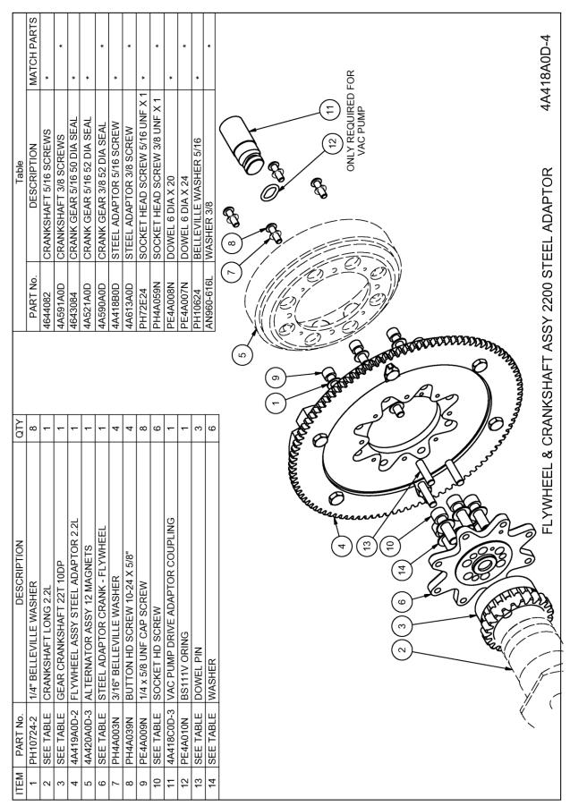
Figure 10 - Crankshaft to Flywheel Assy from S/N 2732
