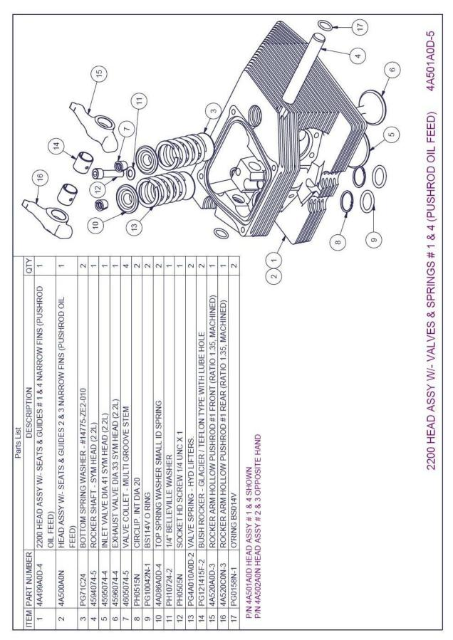
Figure 2 - Cylinder Head Assy
