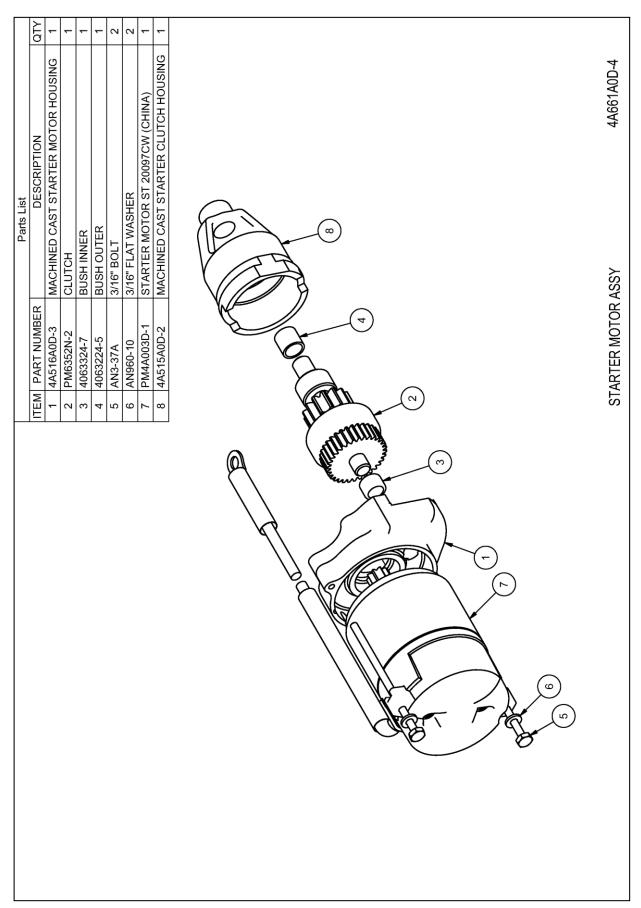
Figure 16 - Starter Assy Cast Housing
