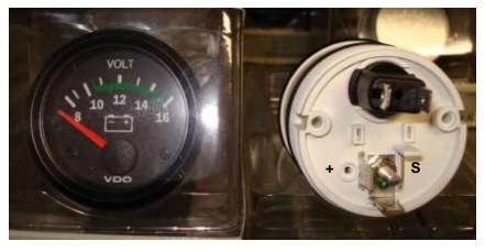
**Figure 21. Voltage Gauge Connections**
