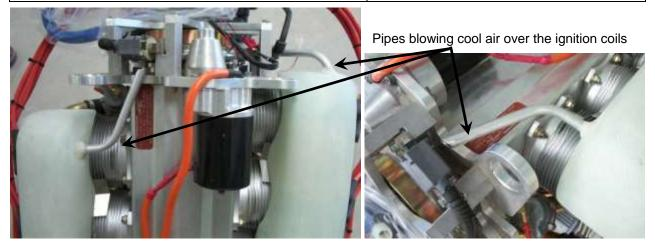
Figure 51. Coil Cooling Detail
