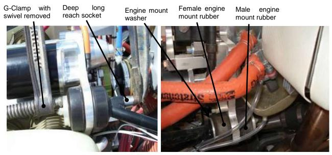
Figure 41 Upper & Lower Engine Mount Detail
