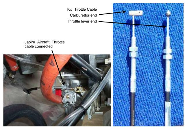
Figure 46. Control Connections to Carburettor
