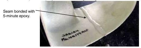
Figure 52. Ram Air Duct Front Seam
