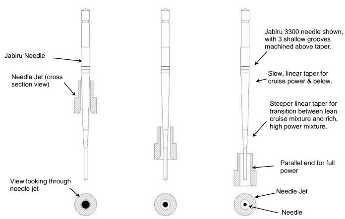
Figure 32. Needle Jet (Jabiru Needle)
