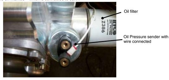
Figure 19. Oil Pressure Sender
