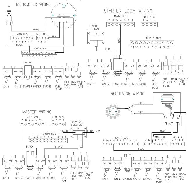
Figure 63. Wiring Details
