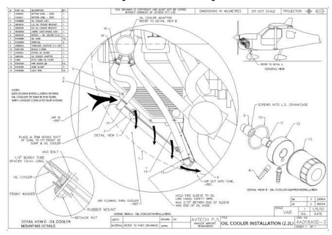
Figure 55. Oil Cooler Installation
