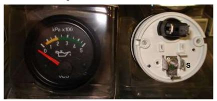
Figure 20. Oil Pressure Connections
