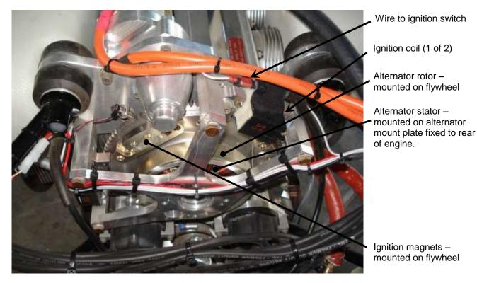
Figure 9. Ignition & Alternator Detail
