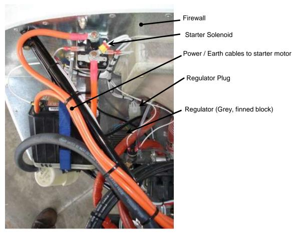
Figure 11. Electrics Installation to Firewall
