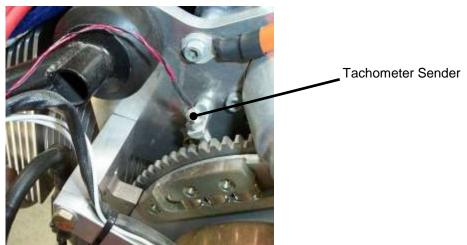
Figure 15. Tachometer Sender Installation
