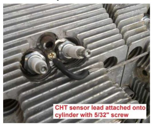
Figure 24. CHT sensor between plugs
