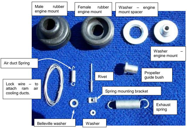
**Figure 40. Engine Accessory Pack Contents**
