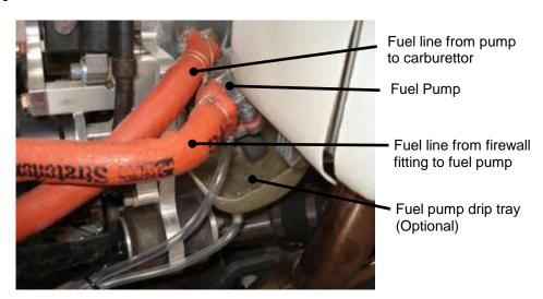
Figure 28. Mechanical Fuel Pump
