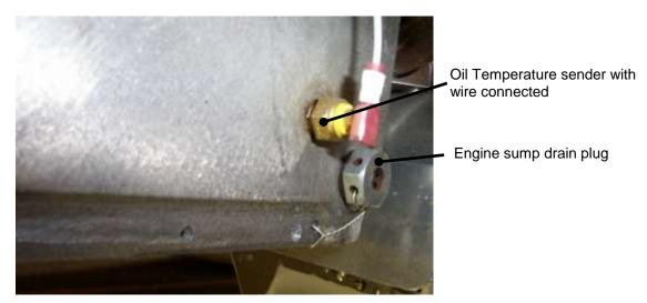
Figure 17. Oil Temperature Sender
