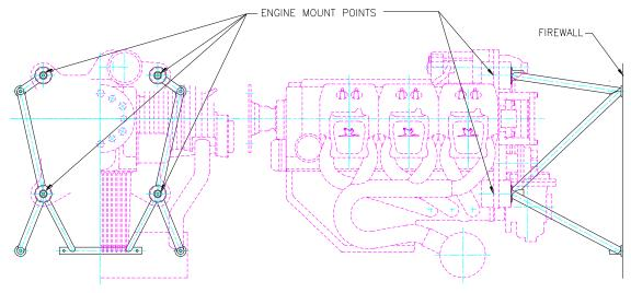
**Figure 4. Engine Mount Point Locations**
