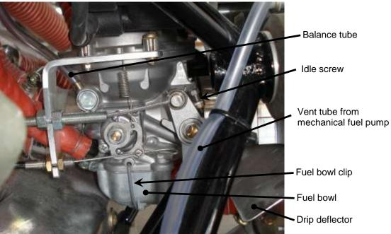
Figure 29. Carburettor Installation
