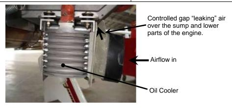
Figure 54. Oil Cooler Duct Design
