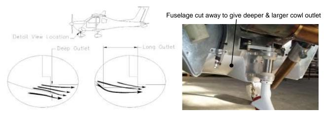
Figure 58. Cowl Outlet Geometry
