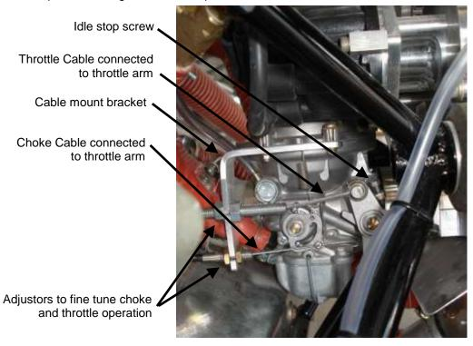
Figure 7. Choke and Throttle Connections to Carburettor
