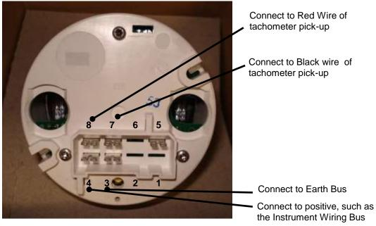
**Figure 16. Tachometer Connections**
