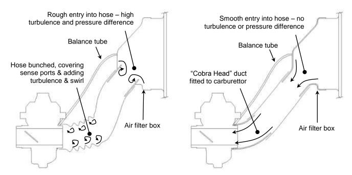
Figure 33. Air Intake Connections
