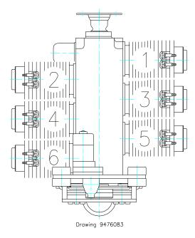
Figure 2. Cylinder Firing Order
