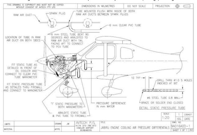
Figure 60: Cooling pressure measurement.
