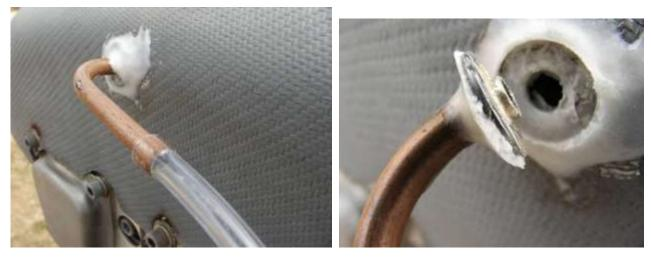
Figure 61: Ram Air duct pressure tapping.
