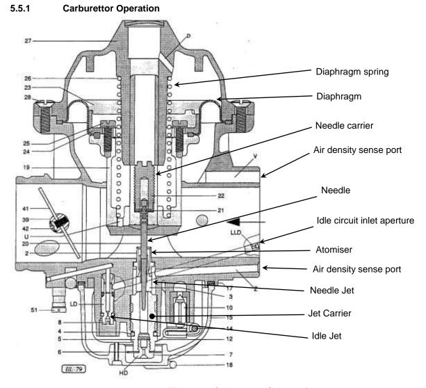
Figure 31. Carburettor Schematic
