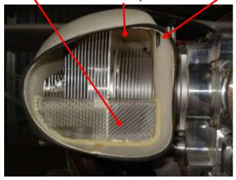
Figure 50. Front-On View Into Ram Air Duct
