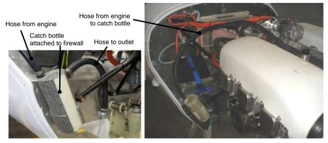
Figure 8. Crankcase Breather Installation
