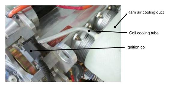
Figure 13. Ignition Coil Cooling Tube
