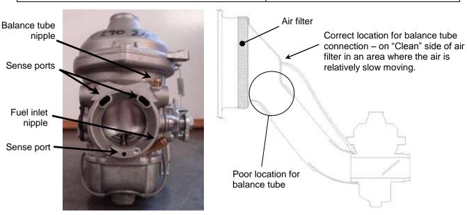
Figure 30. Carburettor Intake & Balance Tube Detail
