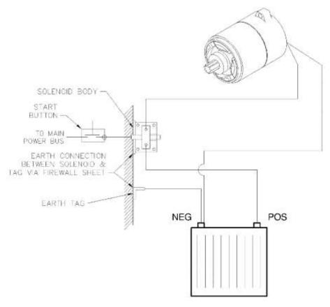
Figure 14. Starter Wiring Details
