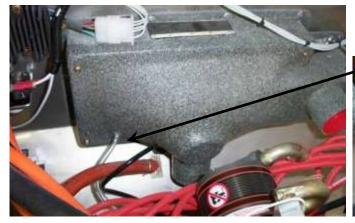
Balance tube connecting filtered side of air mixer box to nipple on carburettor.
