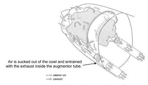
Figure 62. Augmentor Exhaust System
